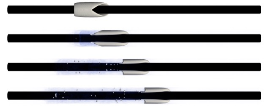
An example of the bubble propagation through the concentric annular pipe at different timesteps. 2
